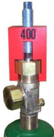
Stripped Valve Stem Clamping Device:
