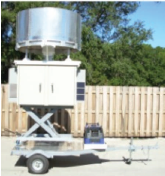
Ilustración 2.48 Vesper Fixed-beam. Vertical Profile Bird & Bat Radar
